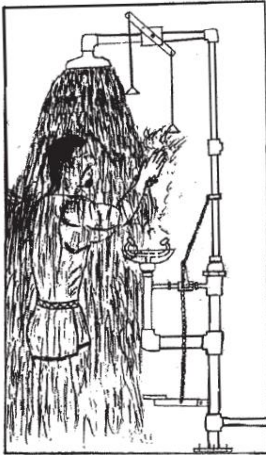
Figure 22: Emergency Shower And Eye Wash Fountain
