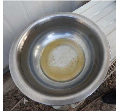
Figure 1: Sediments in Water drawn from bulk supply area (for Donkey Carts and Trucks in Bentiu Water Utility)
